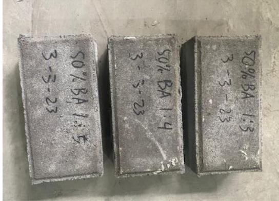
Gambar 2 Benda Uji Paving Blok
