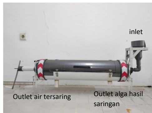
**Gambar 8 Inlet Air Tercemar (a), Outlet Air Tersaring (b), Outlet Alga Hasil Saringan (c)**
